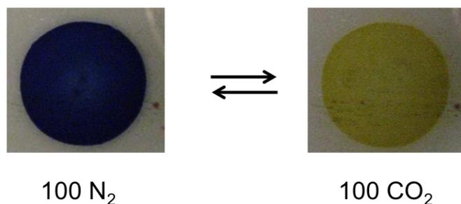
Figure 1. Water based CO<sub>2</sub> sensor colour variation at 100% Nitrogen and 100% CO<sub>2</sub> atmospheres.
