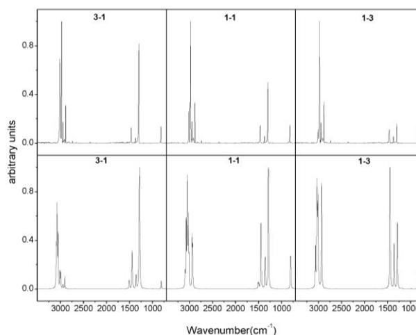
Fig. 2. Comparison of experimental (top) and calculated spectra in the mid-IR for three of the mixtures studied in this work with the indicated CH<sub>4</sub>:C<sub>2</sub>H<sub>6</sub> ratio
