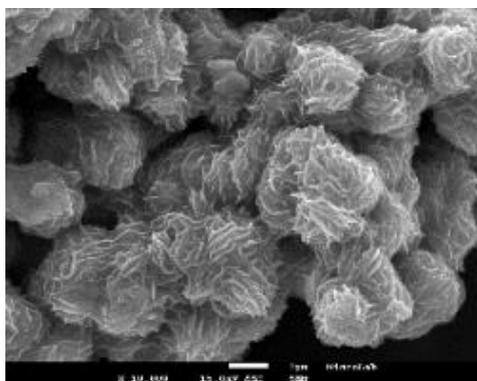
Fig. 1 – SEM image of a Mo heterogeneous catalyst
