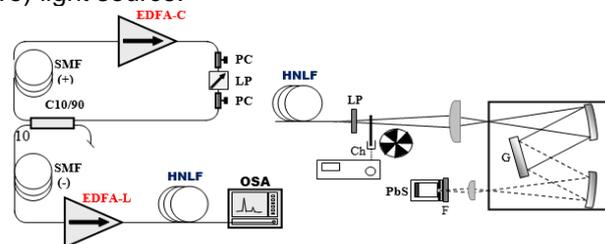
**Figure 1.** Experimental setup for the supercontinuum generation.
