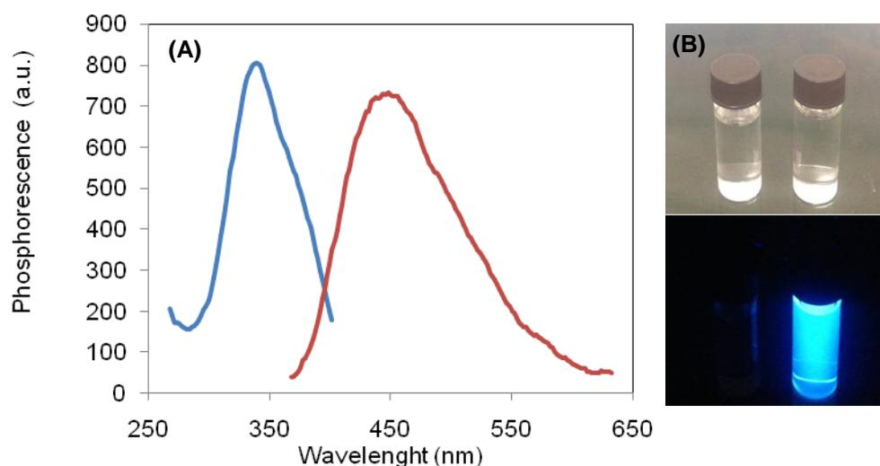
Figure 1. (A) Phosphorescence emission and excitation spectrum. (B) Photographs of Cdots solutions under visible light (right) and UV beam of 365 nm (left) in comparison with only water
