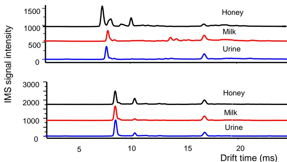
Figure 1. IMS plasmagrams of urine (blue line), skimmed milk (red line), and honey (black line) samples spiked with chloramphenicol at 50  $\mu\text{g L}^{-1}$  using IAC-DLLME and MIP-DLLME before IMS measurement.
