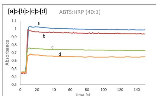
b.- Working with low concentrations of ABTS it is possible to obtain a transient signal (fig 2).
